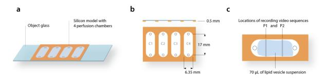
Figure 2: (a) Scheme of the perfusion chambers. (b) Silicone model with four perfusion chambers (C1–C4). The side view is given in the figure and the depth of the chambers is 0.5 mm.
