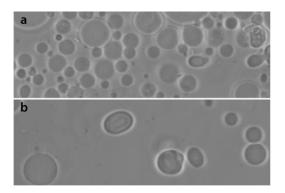
**Figure 1**: Micrographs of two vesicle populations with different vesicle densities in solution. Vesicle abundance is higher in (a) than in (b). The lower abundance of vesicles (b) is preferred for better performance of the computer vision algorithms.
